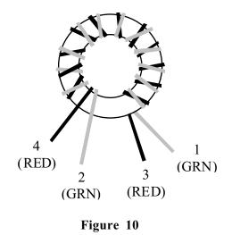
Install T1 vertically on the PC board as indicated by its outline near the back edge of the board. Insert the red and green leads into their numbered holes (see lead numbering above).
