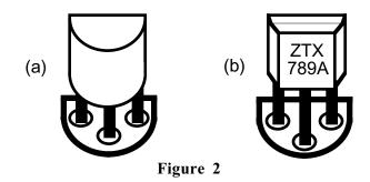
Locate the two 2N7000 transistors. Install these at Q2 and Q3 as shown in Figure 2a. Q2 is near the center 2-D fastener on the right edge, and Q3 is near the microcontroller, U1. The flat side of each transistor should be aligned with the flat side of its component outline.
